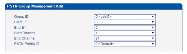
In the above figure, as start E1 is the same with end E1, only one E1 port is used in the PSTN group and you need to set start channel and end channel.
