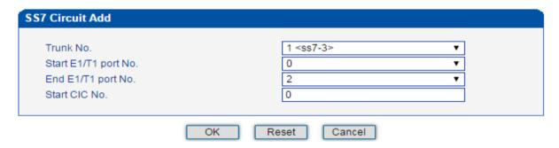
If multiple E1/T1 ports are involved, it defaults that all the 32 channels of each E1/T1 port involved are used by the SS7 trunk.
