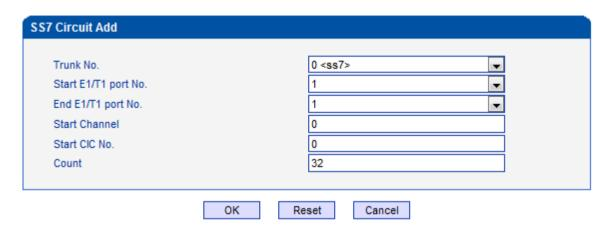
As there are 32 channels (from 0 to 31) for one E1/T1 port, so the value for **Count** is 32. When start E1/T1 port is the same with end E1/T1 port, it means only one E1/T1 port is connected to the SS7 trunk.
